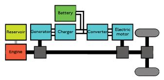
Fig. 4. Power split combined hybrid powertrain
