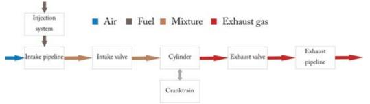
Fig. 1. Block diagram of the engine model
